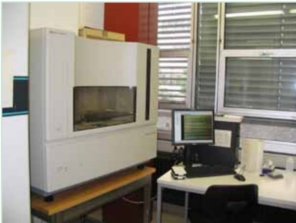
A 96-capillary DNA sequencer from Applied Biosystems for high-throughput DNA sequencing. The 3730xl instrument takes up stacks of 96-well microtiterplates containing sequencing reactions with four different fluorescent terminators, one for each of the four bases in DNA. The sensitive detection of the fluorescent signals allows read lengths up to more than 900 bases per read.
