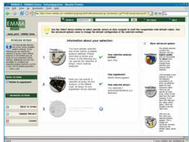
Fig. 2: The EMMA software provides a user friendly interface for the configuration of individual data analysis pipelines. The screenshot shows the pipeline configuration dialog that allows a step by step creation of reusable data analysis workflows.
