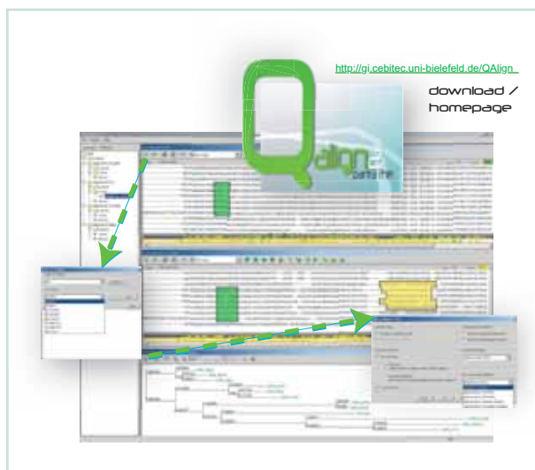
Fig. 3: QAlign2 - panta rhei: a tool to automatically generate multiple alignments (middle of left border) and to visually control the results (top-right area of the main panel). A guided editing function allows changes done by hand (marked boxes), and phylogenetic trees can be inferred on every alignment layout (bottom).
