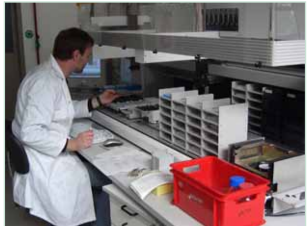
A robotic device to load the samples for MALDI-TOF (Matrix-Assisted Laser Desorption Ionisation - Time Of Flight; a specific type of mass spectroscopy) analyses onto the target support arrays. The samples are spotted onto a metal support as an array of 96 or 384 spots. The results allow for example the identification of proteins present in the samples on the basis of molecular masses of peptides.
