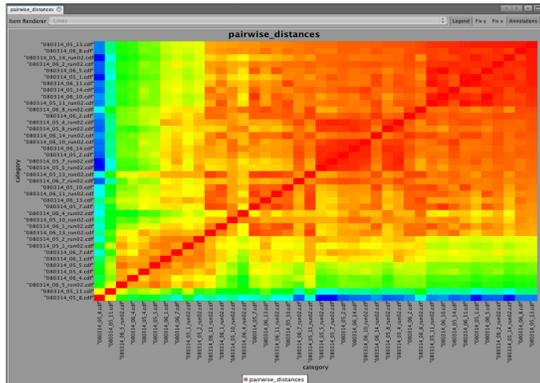
Figure 2: Inverse Visualization of pairwise distances as similarities. Blue color indicates a low similarity between chromatograms, while red indicates a high similarity. Similarities were calculated using the partitioned dynamic time warping (DTW) algorithm with automatically determined anchors on GC-MS data from an experiment that examined the impact of CO<sub>2</sub> concentration on the biomass production of common wheat [2].
