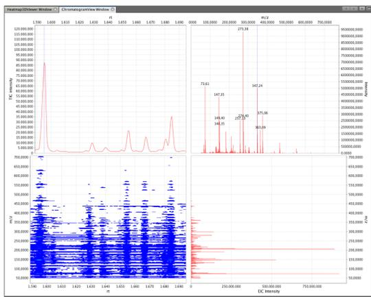
Figure 1: Screenshot of the ChromAUI application, showing the GC/LC-MS heatmap view at the bottom left. Above, the total ion count (TIC) is displayed. In the upper right hand panel the mass spectra for selected scans are shown. The panel on the lower right hand side displays the cumulative ion channel intensity.
