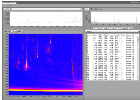
Figure 4: Interactive heatmap view within ChromAUI, clockwise from bottom left, showing a section of a GCxGC-MS chromatogram heatmap in a custom color scheme with peak markers, the total ion count for the modulations, the mass spectrum of selected peaks, and the peak list of the chromatogram.
