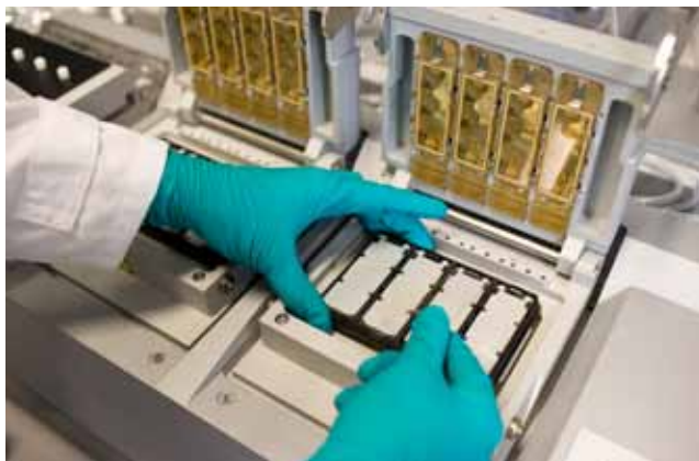
Figure 3: Microarray hybridization station for automated and reproducible microarray processing in transcriptomics analysis.
