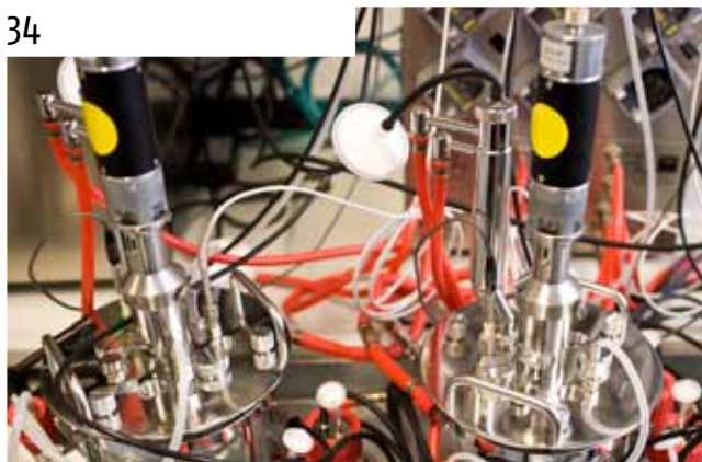
Figure 1: Bioreactor system for parallel operation. The fermenter system is capable of controlling temperature, pH, pO_2 , agitation speed, gas composition etc. in different culture vessels independently.
