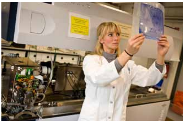
Figure 3: A scientist inspecting a two-dimensional protein gel in front of an opened MALDI mass spectrometer.
