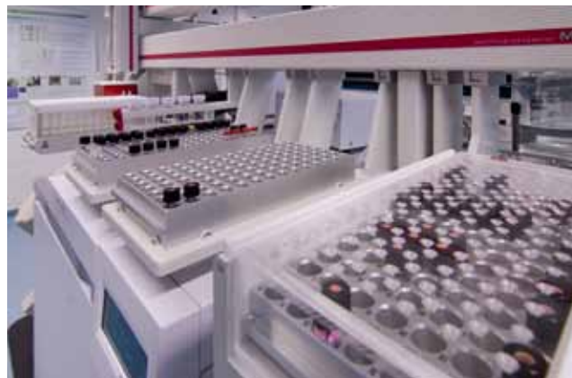
Figure 4: Two-dimensional gas chromatography with time-of-flight mass spectrometer (GCxGC-TOFMS) equipped with a multifunctional autosampler and sample preparation robot. The GCxGC-TOFMS system allows high resolution metabolomics analysis.
