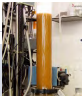
Mass production of algae in a photo-bioreactor with central illumination
