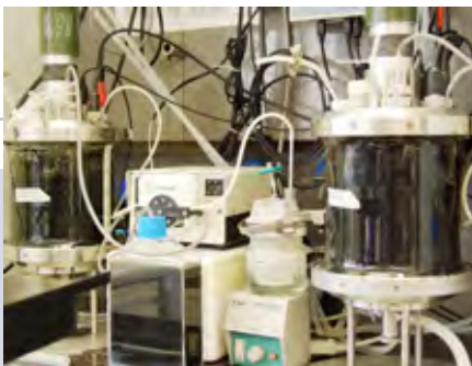
Two-stage continuously operated biogas reactor
