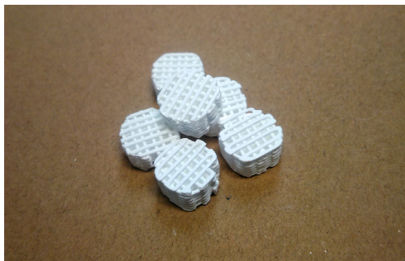
Figure 3. 3D-printed ceramic monoliths for catalysts immobilization.
